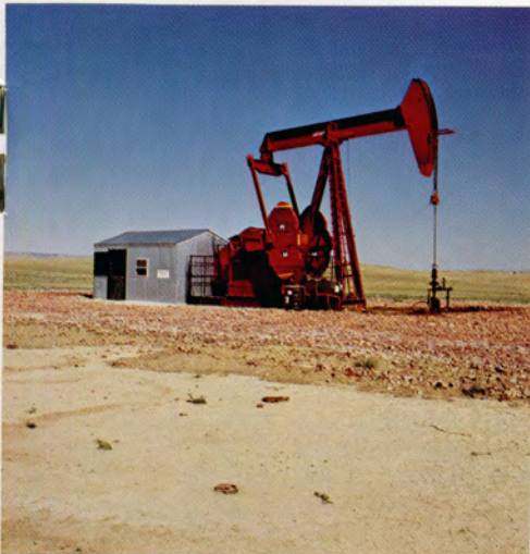
LUFKIN C-456D-305-120, Reading & Bates Petroleum Co., Campbell County, Wyoming.
