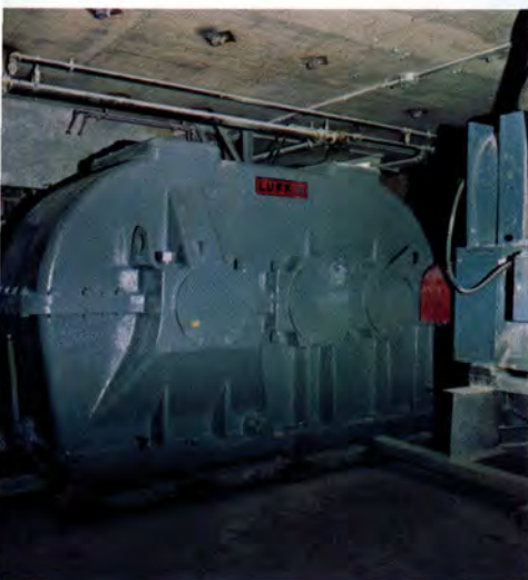
LUFKIN D340C reducer powers the buckets unloading coal barges for the Union Railroad Company from a platform engineered and designed by Heyl & Patterson, Inc., Pittsburgh, Pennsylvania
