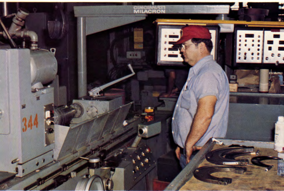
Cincinnati 10" X 60" 380 Plain Grinder shown here in the process of grinding an industrial gear shaft
