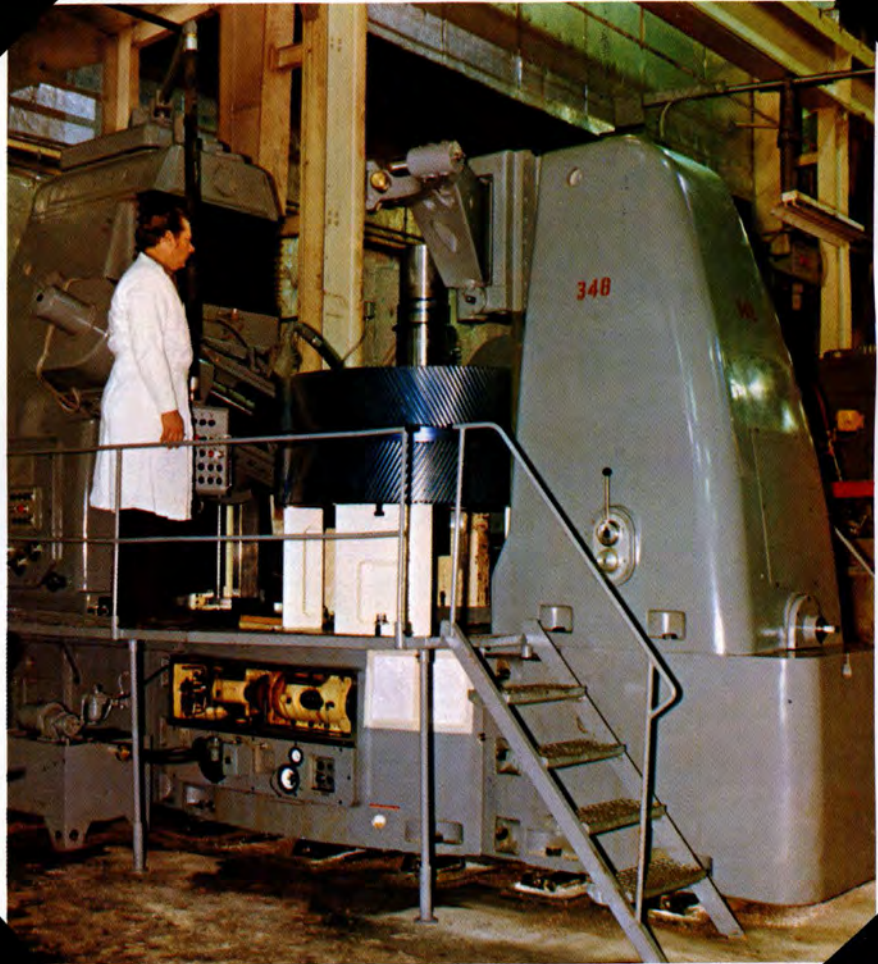
This large hobbing machine, especially designed for extreme accuracy, is a new addition to production facilities.
