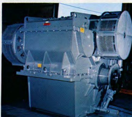
LUFKIN Model RS3622 marine gear with an input of 865 rpm reduced to 174 rpm will produce 2575 horsepower for use in a Great Lakes vessel.
