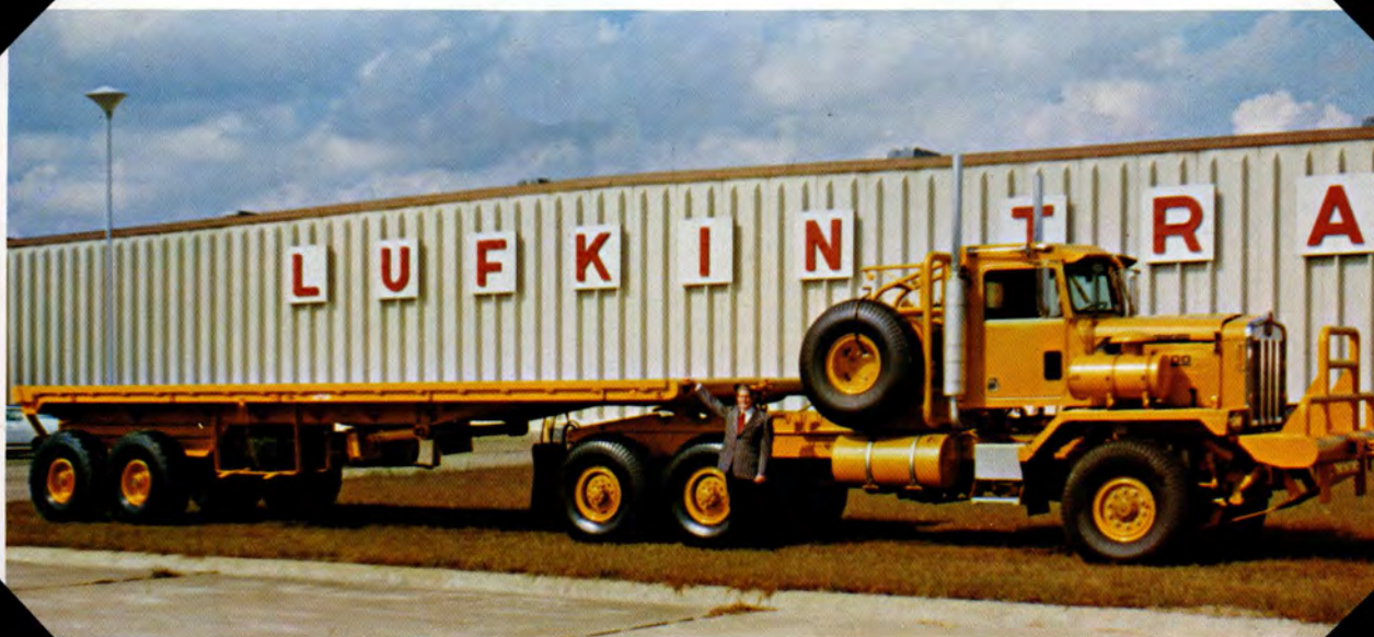
LUFKIN trailer specially designed for desert-based oil field operations. The trailer bed is 7½ feet from the ground.
