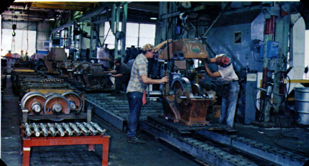
The pumping unit gear reducer is assembled, inspected, and sent to the final assembly area where it is mounted on the pumping unit structure.
