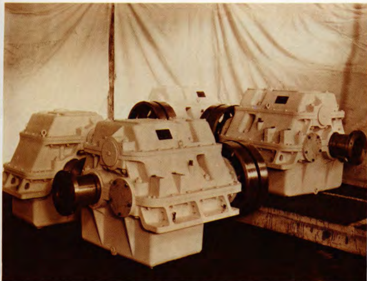
LUFKIN marine gears prior to shipment to shipyards around the country for installation in LST landing craft, Navy destroyers, and Army cargo vessels during World War II.
