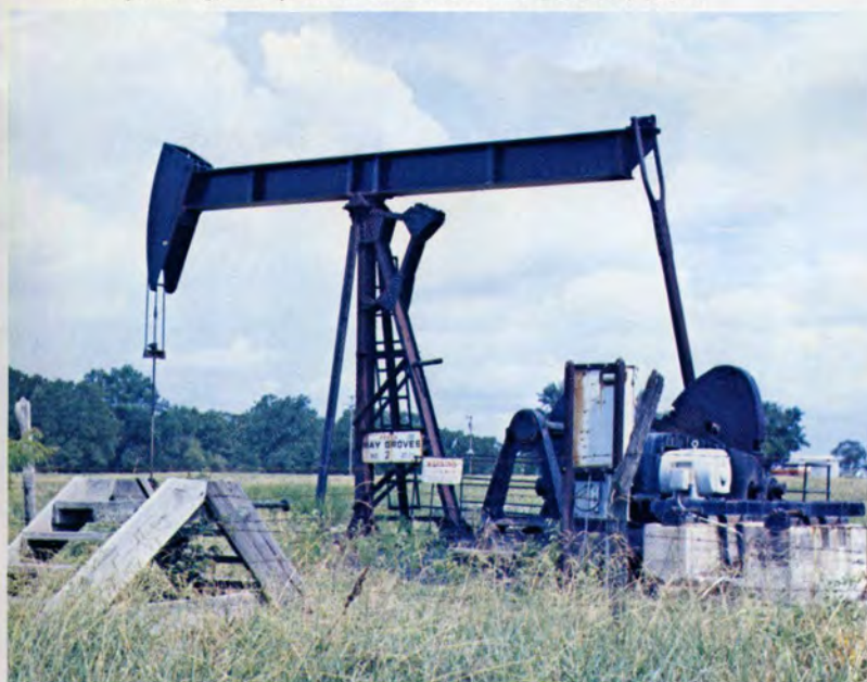
LUFKIN 5½ worm gear unit complete, Humble Oil Company, Seidel, Texas, shipped late August, 1929. It is still operating; this photo was made in the summer, 1977.
