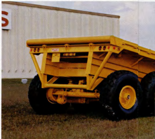
LUFKIN mounted a heavy duty pipe bumper, a pipe grill guard, and a 1/2" belly pan to offer maximum protection for off the road operations
