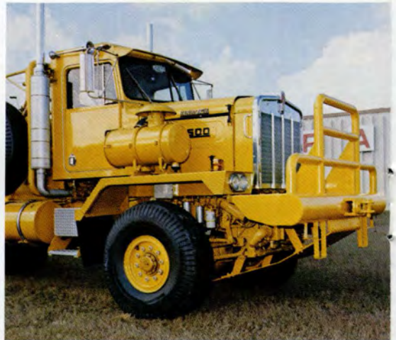
LUFKIN mounted a heavy duty pipe bumper, a pipe grill guard, and a 1/2" belly pan to offer maximum protection for off the road operations
