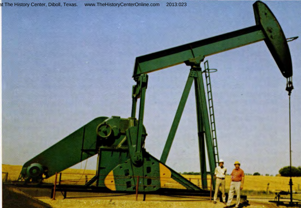
LUFKIN C-912D-305-168 Unit, Texaco, Ascheberg, Germany
