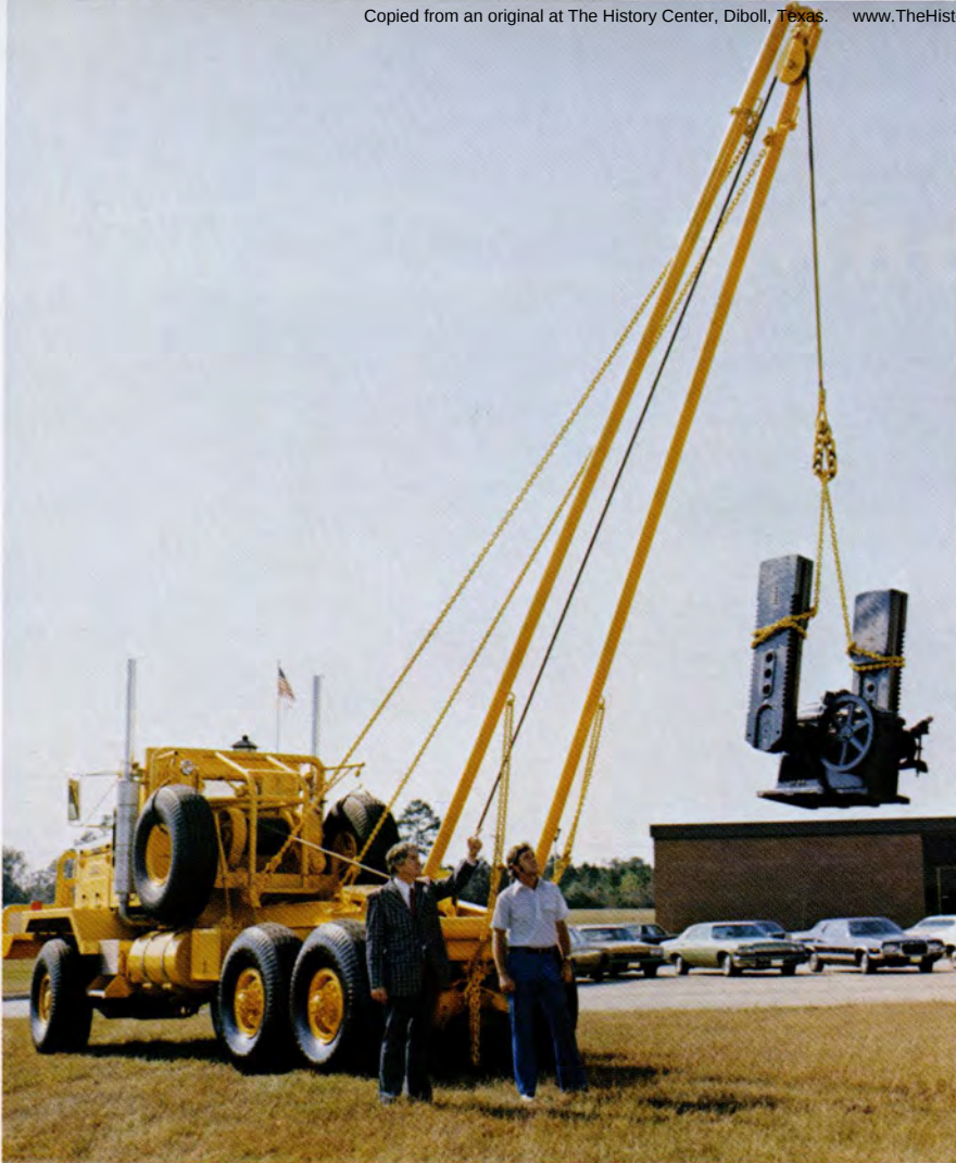
The 24-foot gin poles pick up a LUFKIN 40D gear box assembly as it prepares to load a "self-loader" float. LUFKIN mounted "I" beam runners, a fifth wheel, tool tray, tool box, gin pole pockets, utility spot light on the headache rack, stay chains, gin pole assembly with snatch block, draw bar, and rolling tail pipe atop the bed of the truck
