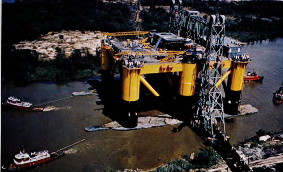
Traversing through the Intracoastal Canal, on way to sea trials, the Zapata Uglund had to submerge partially to clear drawbridges on the waterway
