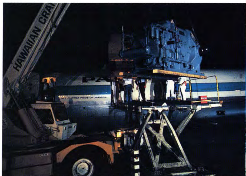
LUFKIN Model NT720BHH High Speed Reducer, Rated 1500 HP, Ratio 44.95:1, 3600 RPM Steam Turbine Input to 80 RPM Sugar Cane Crusher. This Reducer was sold to Bitco Pacific Corp., Honolulu, for Oahu Sugar Co., Waipahu, Hawaii. This gear, (actual scale weight was 26,860 pounds) was air-freighted by Pan American 707 from San Francisco to Honolulu in five hours.
