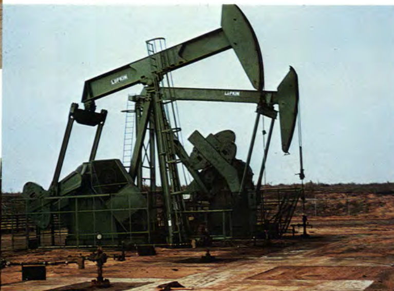
LUFKIN C-912D-356-144 and LUFKIN M-921D-304-144 Units, Chanslor Western Oil & Development Co., Torrance, California.
