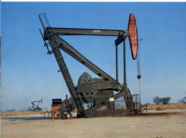
LUFKIN M-912D-305-192 Unit, Tenneco Oil Company, Greeley, California.
