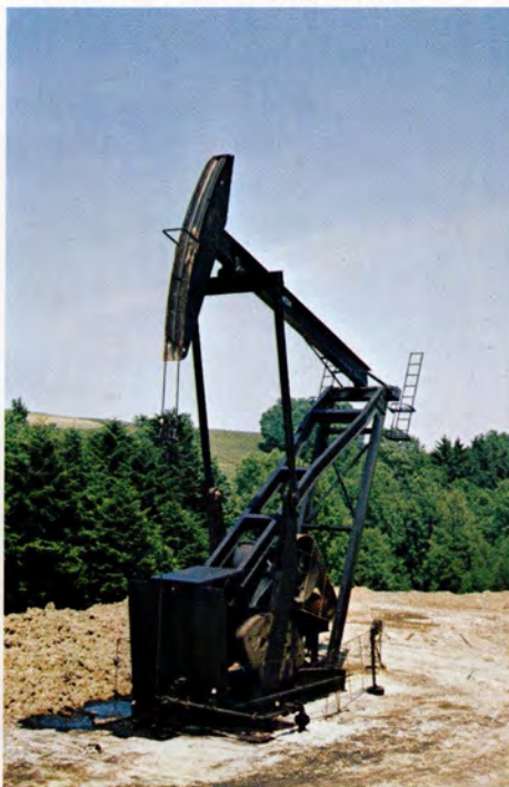
LUFKIN M-1280D-427-216 Unit, Mobil Oil Austria A.G., Kremsmunster, Austria
