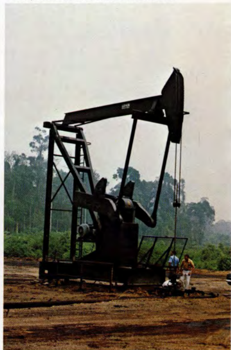
LUFKIN M-228D-256-100 Unit, P.T. Caltex Pacific Indonesia, South Balam Field, Central Sumatra, Indonesia
