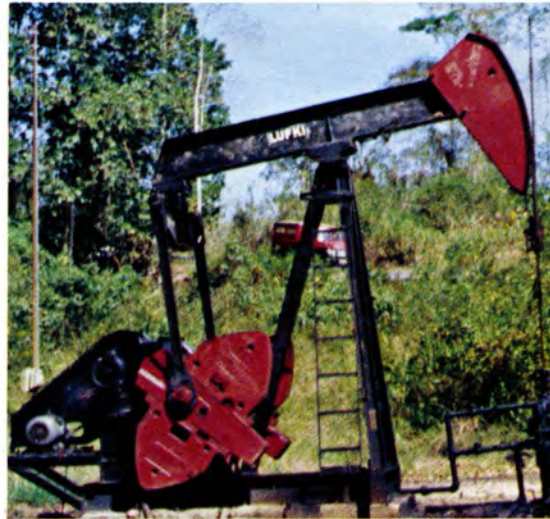
LUFKIN C-114D-143-64 Unit, Trinidad- Tesoro Petroleum Company, Ltd., Coora Field, Trinidad.
