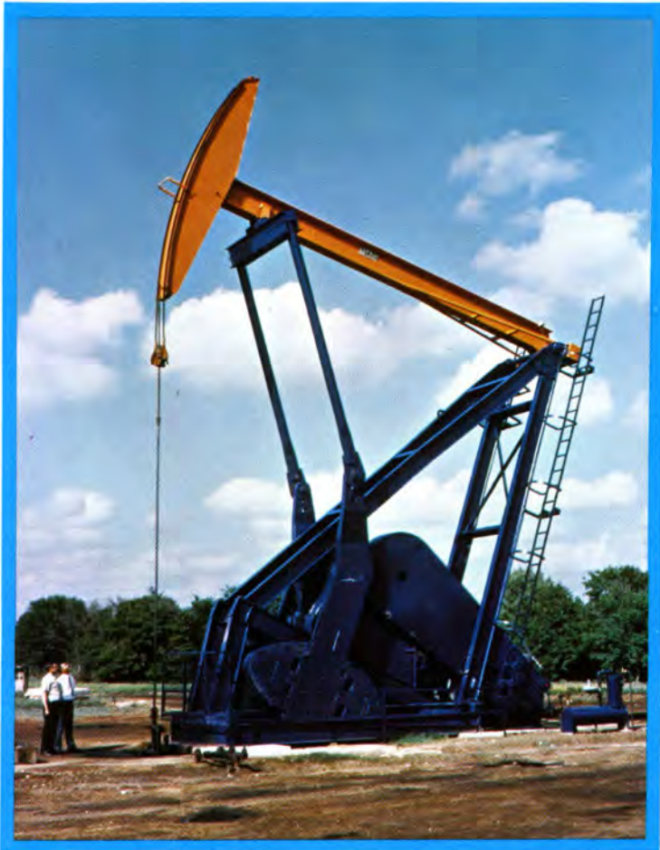
LUFKIN M-1280D-427-216 UNIT, DRIVEN BY A LUFKIN H795 ENGINE
