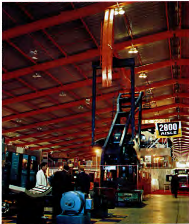
DOMINATING the east end of the Tulsa Exposition Center was the largest crank counterbalanced pumping unit in the world. In operation at the show, the unit's head nearly reached the roof of the 10½-acre building at the top of its stroke.
