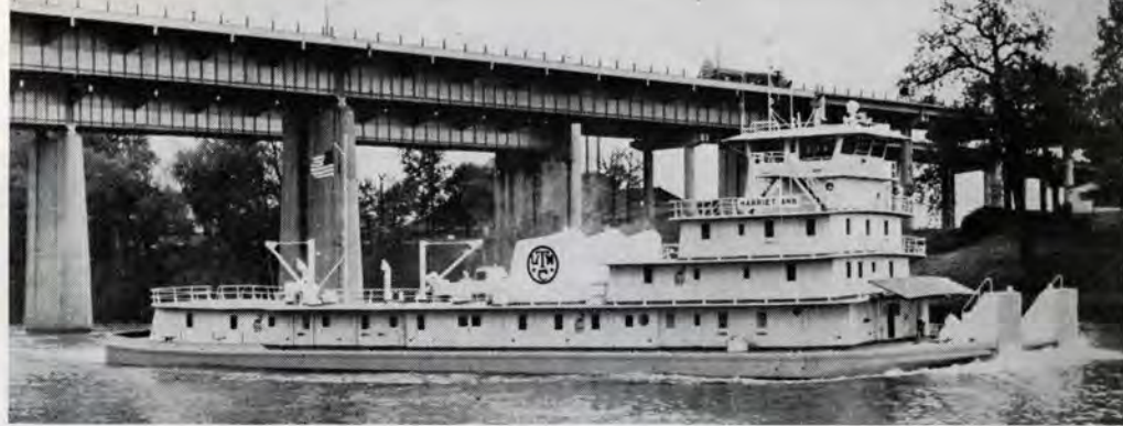
THE HARRIET ANN , 198 feet long, 50 feet wide and 11½ feet deep handles approximately 45,000 tons on a down-river trip
