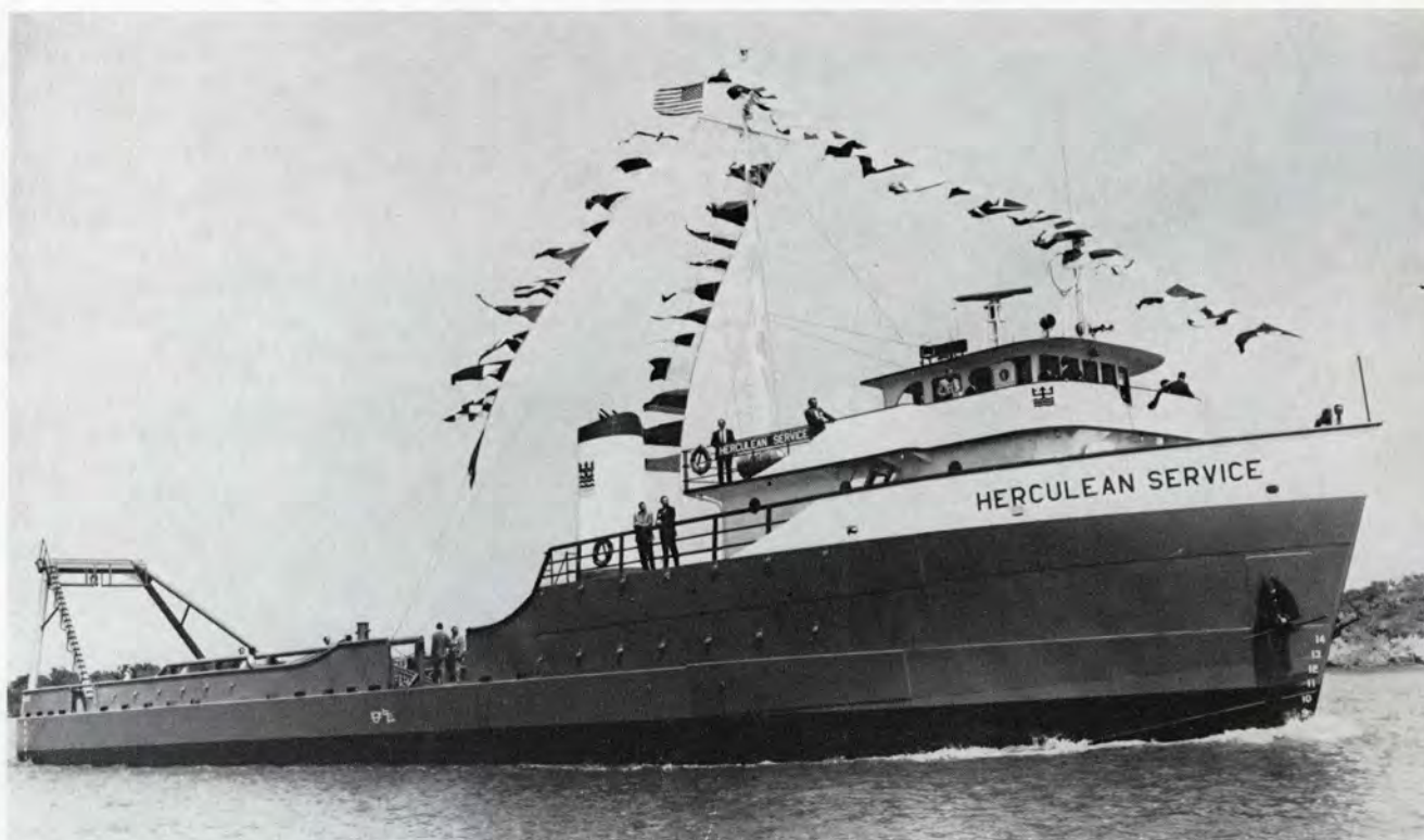
THIS two-speed, triple-screw vessel is one of the first to be specifically designed for offshore tug-supply service. Christened May 12, Herculean Service was added to the Zapata Marine Service fleet.
