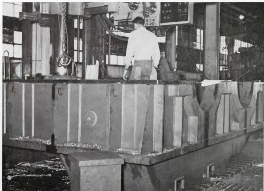
5. LUFKIN's American Openside Tape Drilling machine is programmed to position itself to drill precisely various hole patterns. This machine has the capacity to drill a piece 20' long, 7' wide and 9' high. The 16-foot wide HDL 6640 gear box was too large to be drilled at one setting. One half the box was drilled and then turned for the other half to be drilled
