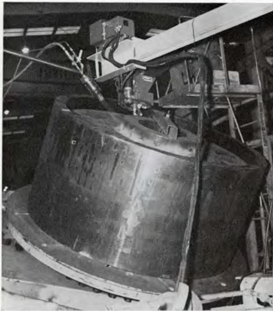
3. THIS photograph shows the center sub-assembly composed of the hub and web plate
