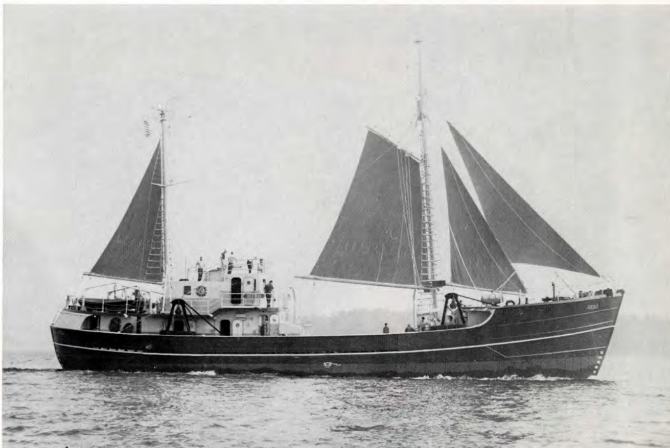
LOOKING akin to a New England trawler, HERO, was constructed for work in the icy waters of the Antarctic. Her conservative sails are rigged for use in heavy weather.
