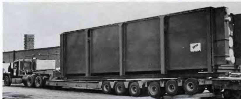
LUFKIN 3-axle lowboy with LUFKIN 3-axle dolly carrying 190,000-lb. heaters , an example of Hicks' specialized hauling
