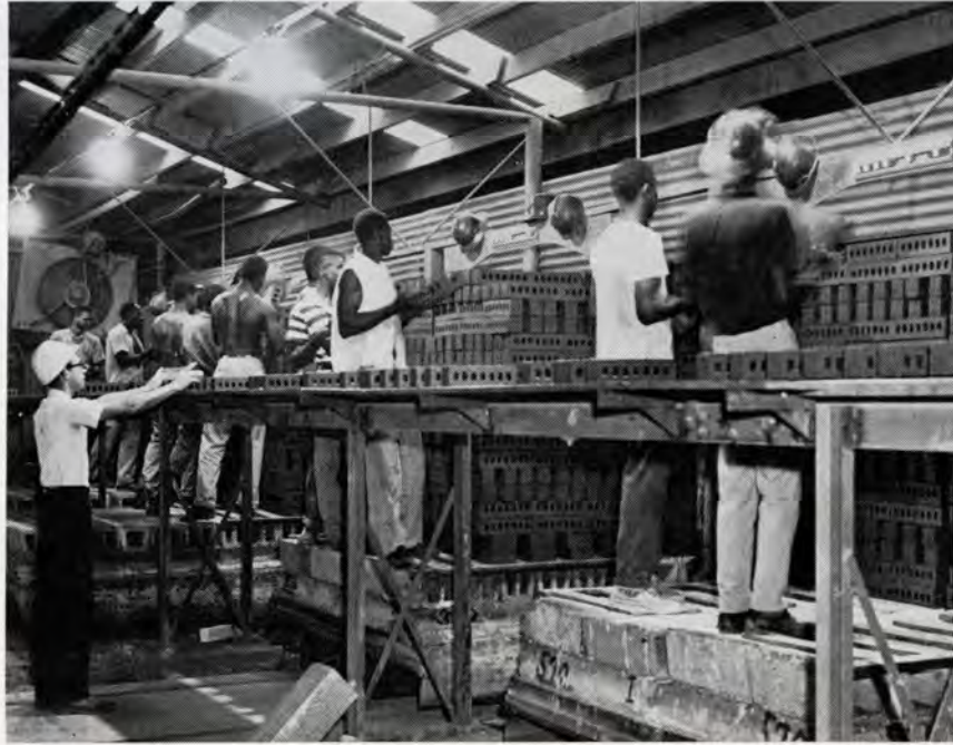
HACKERS are transferring unfired brick to kiln cars. This is only one of two times that brick are handled by hand
