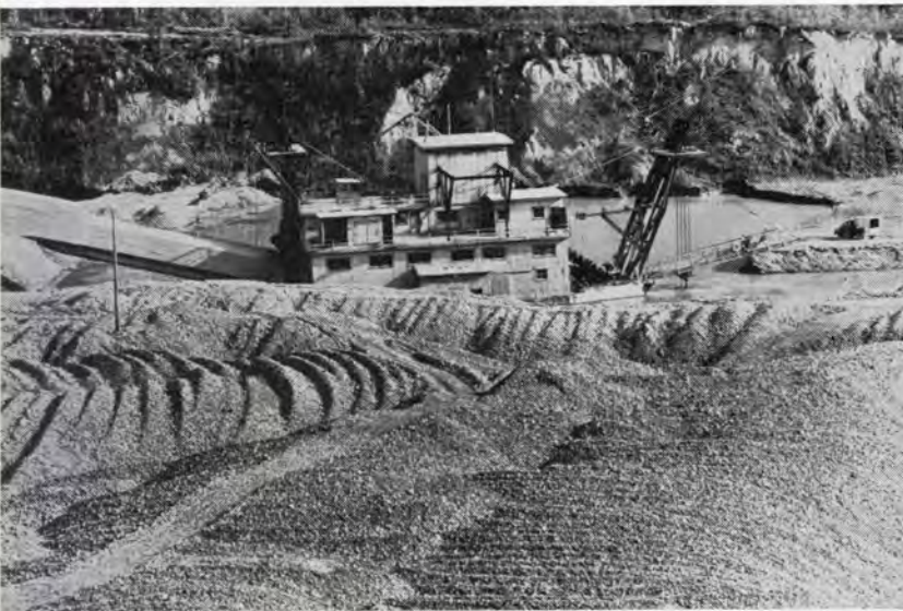
LARGE gold dredge gobbles up river bed down to bed-rock, goldplating sluice boxes with nuggets and flour gold.
