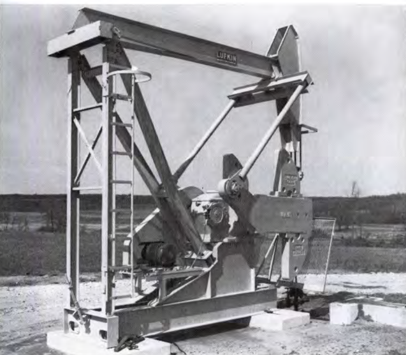
TYPICAL LUFKIN M-114D-143-86 Unit with two-point suspension base, set on pre-cast blocks, with a sand pad, driven by 15 HP motor. The simplicity and economy of this type base results in easier moves to other locations
