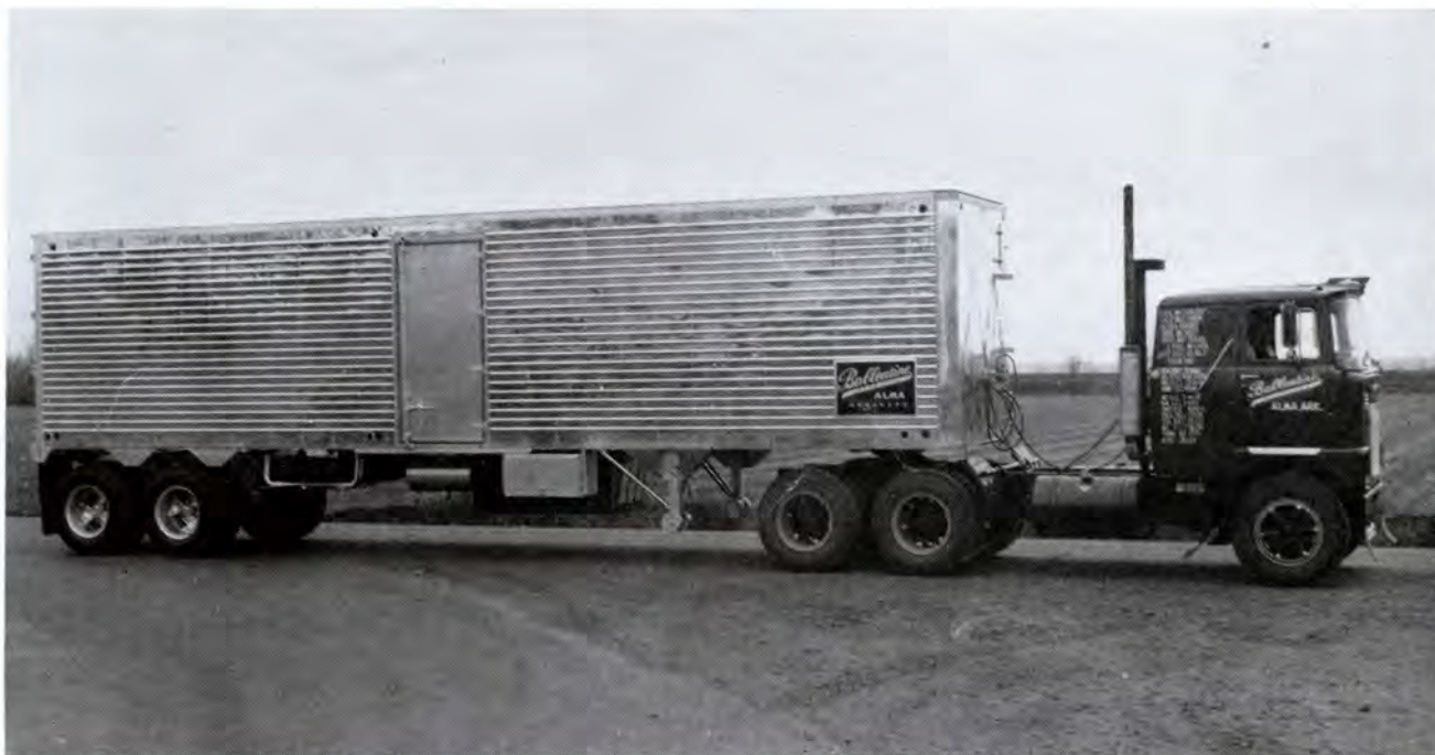
ONE of Ballentine's new LUFKIN refrigerated vans with foam-in-place insulation
