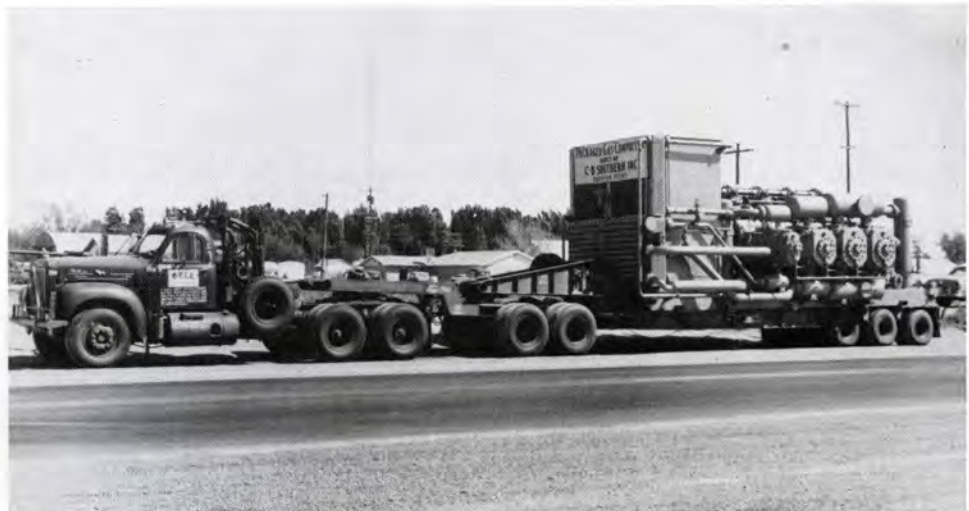
ABOVE are shown two of Bell's lowboys required to move an extraordinarily heavy and cumbersome load.
