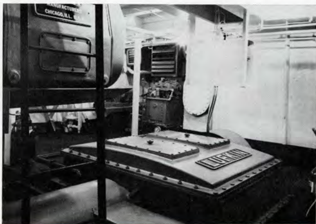
VIEW of completed class 760 YTB tugboat showing Lufkin RS4222 Reverse Reduction gear and the spacious engine room
