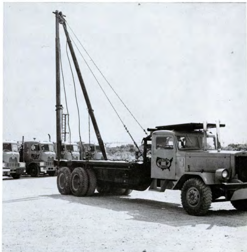
ONE of Dealer's Transit's heavy duty ginpole trucks capable of lifting 35,000 pounds
