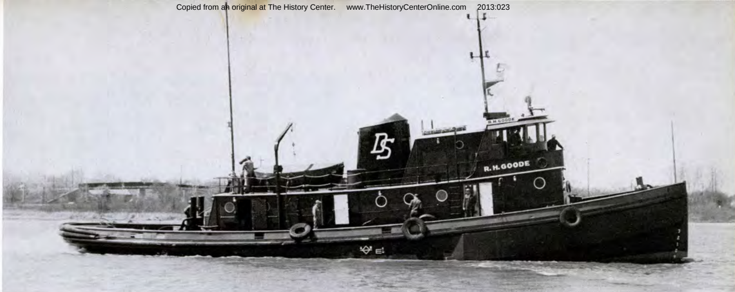
THE R. H. Goode, of Dunbar and Sullivan Dredging Co. of Detroit, was converted from steam to diesel.
