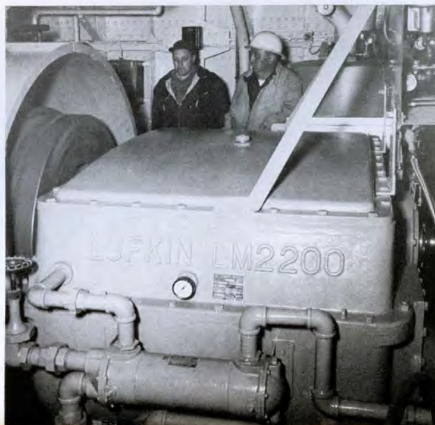
BELOW: This is the Lufkin Model LM 2200 Reverse and Reduction Marine Gear showing Wichita clutch on forward end and air controls on the aft end.
