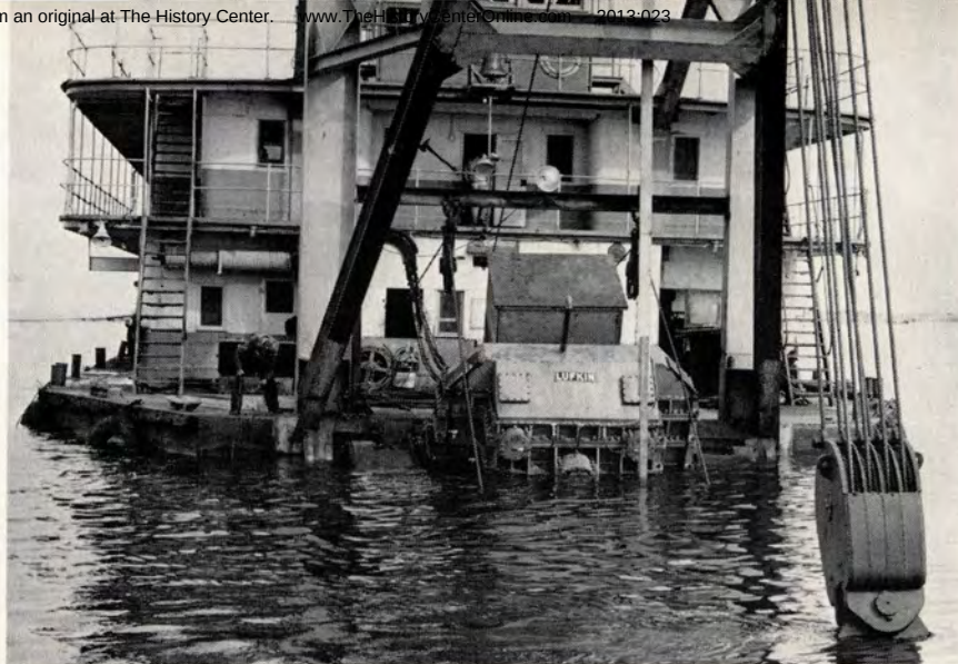
WHEN The Shary is working at full depth, gear is dipped into salt water. Gear box holds 155 gallons of oil, changed every six months
