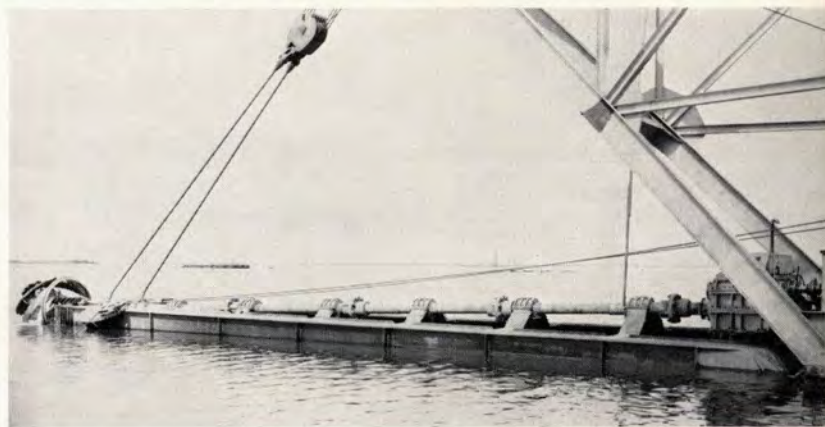
WHEN The Shary is working at full depth, gear is dipped into salt water. Gear box holds 155 gallons of oil, changed every six months
