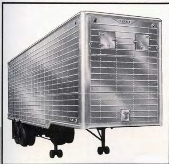
Drop Frame Van with 2270 cu. ft. inside—6 inch or 24 inch radius corners optional.
