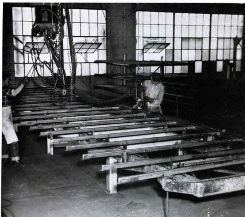
3 THIS is a view of spot welding being done on a sub-assembly side section in the new van shop
