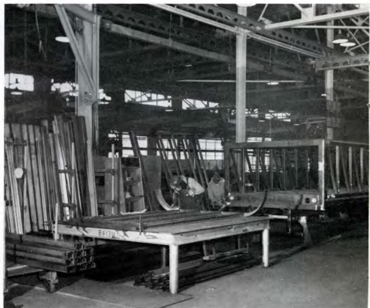
5 WELDING is being done on this sub-assembly which is the front section of a new aluminum van
