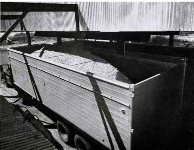
THIS chip-hauling trailer is being loaded by gravity method with chips dropping into van from above
