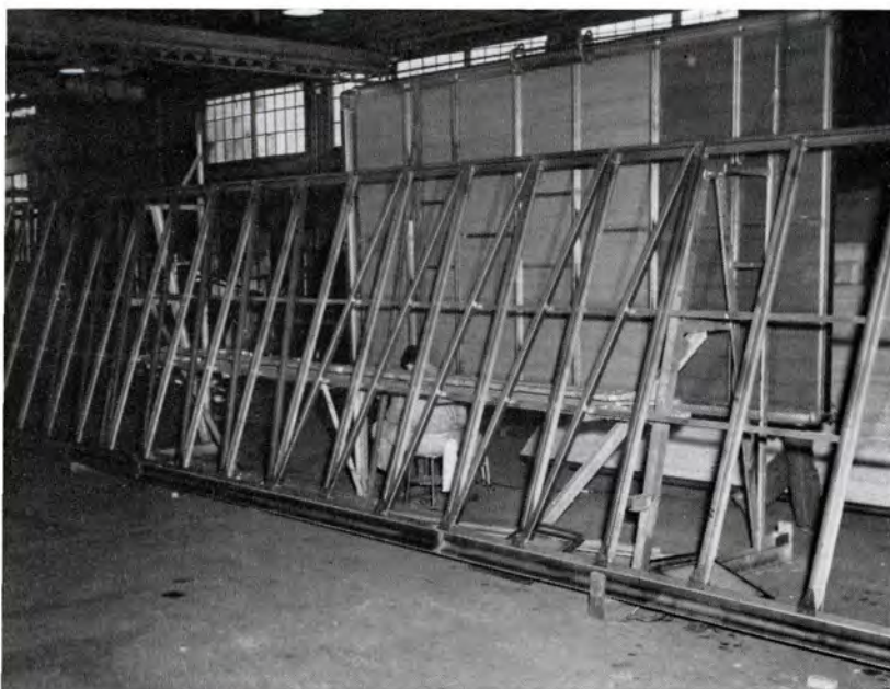
4 THIS is a frame of a trailer side section which is ready for aluminum side sheets to be affixed
