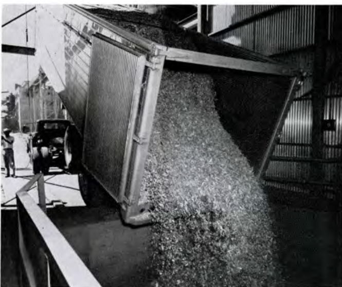
IN A matter of seconds, 30,000 pounds of chips are dumped into a hopper to be used in paper products
