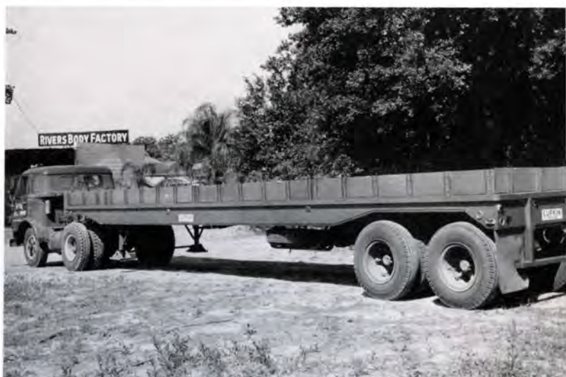
A NEW light-weight bulk fruit trailer has been designed to meet the needs of citrus fruit haulers
