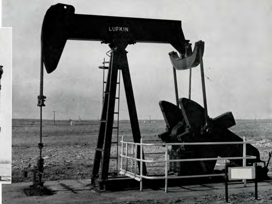
LUFKIN TC-44-15B Pumping Unit in Mid-Burbank Unit, Osage County, Oklahoma.
