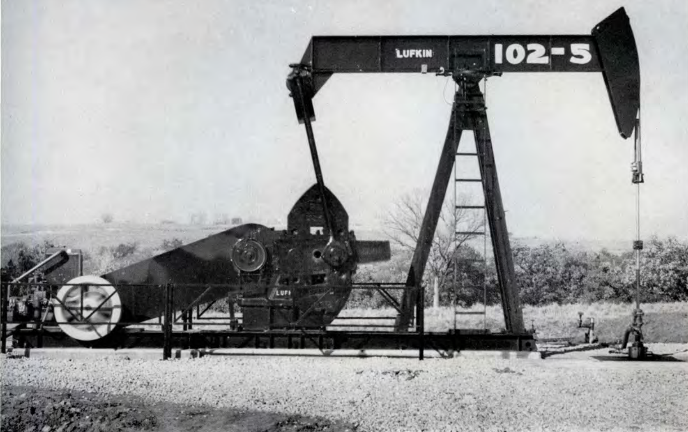
LUFKIN TC-33A-22G Pumping Unit in North Burbank Field, Osage County, Oklahoma
