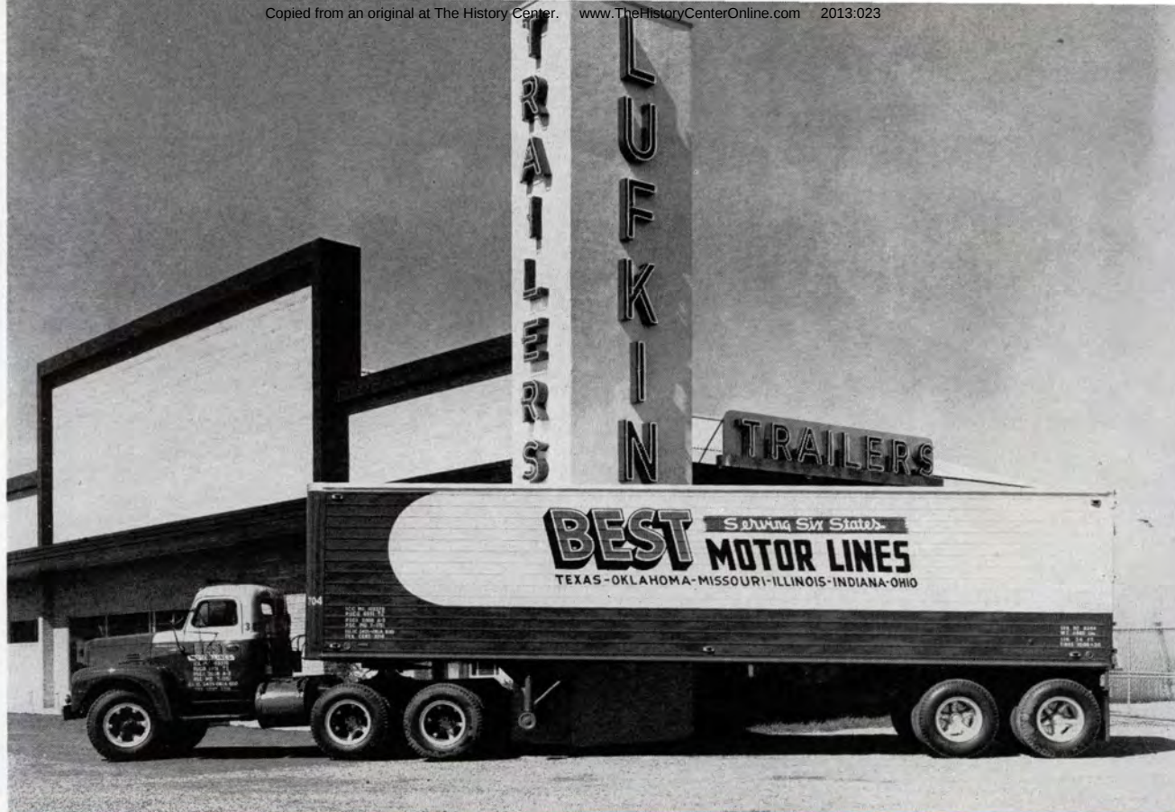
This new square-front, flat-roofed aluminum trailer is the latest model designed by engineers of Lufkin Trailers. This is the first of 48 units ordered by Best.
