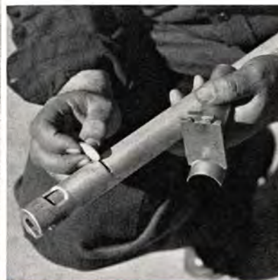
Below left: This inclinometer is made from four instruments—a timer, flashlamp, camera and compass. The unexposed film inserted in the slot records depth readings.
