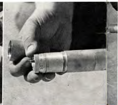
Below left: This inclinometer is made from four instruments—a timer, flashlamp, camera and compass. The unexposed film inserted in the slot records depth readings.
