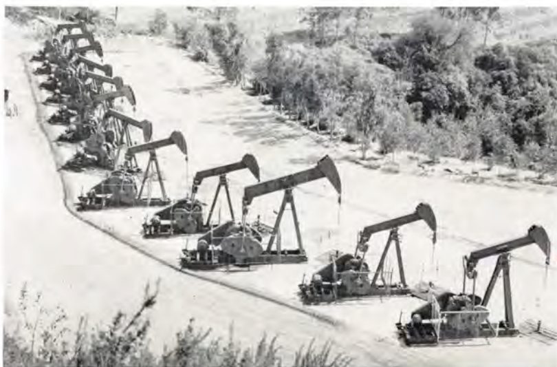
This battery of twelve Lufkin Units stands on the Sanssina Lease of the Union Oil Company of California at Whittier, California. Wells average 4500 feet in depth.
