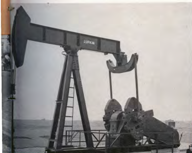
Modern pumping units replace the old pumping jacks on the pilot water-flood.
