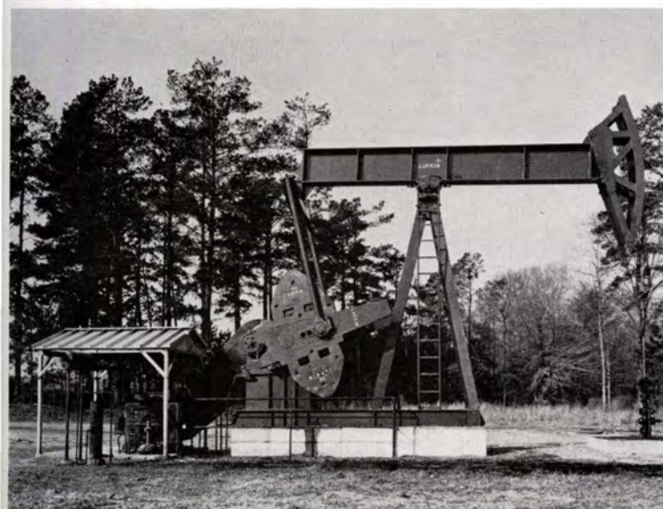
LUFKIN TC-OLC-456DA driven by LUFKIN GSDH engine, The California Company, Houston Smith No. 1, Mallalieu Field, Lincoln County, Brookhaven, Mississippi.
