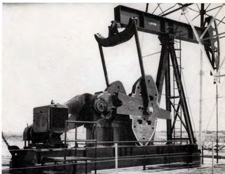
LUFKIN TC-OLL-61B unit, Stanolind Oil and Gas Company, Yarbrough Allen Field, West Texas.
