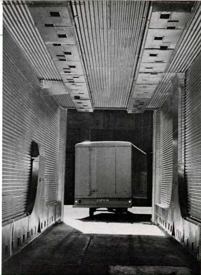
Above right: A NEW BODY, glistening and clean, emerges from Lufkin's giant paint oven. Capable of 750,000 BTU's per hour, the oven is 13½ feet high and 40 feet long. At 190-degree temperature, primer coats can be dried in 60 minutes.
