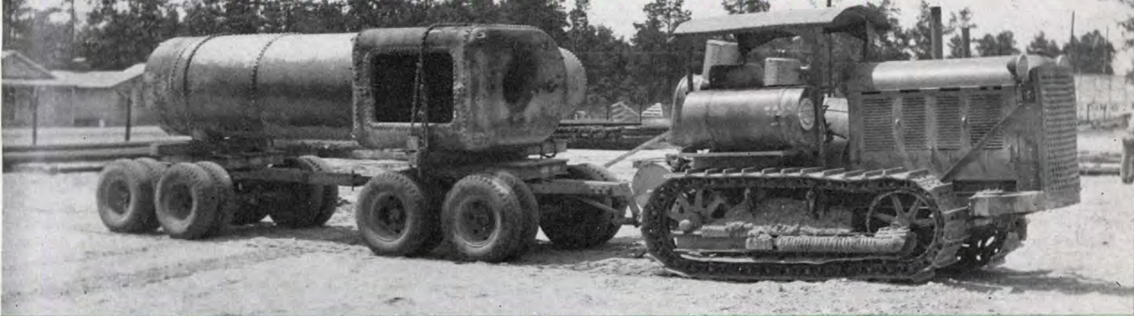
THIS 16-WHEEL TRAILER was built by the Martin Wagon Company before Lufkin Foundry took over the concern. This trailer was used for heavy duty moving that had to be done off the highways in the fields.
