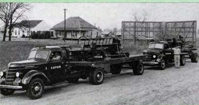
THIS MODEL MIGHT be referred to as a combination oil field bed. It can be used with a single or tandem self loading float, with single or tandem pipe trailer, or as a bed job for local purposes.
