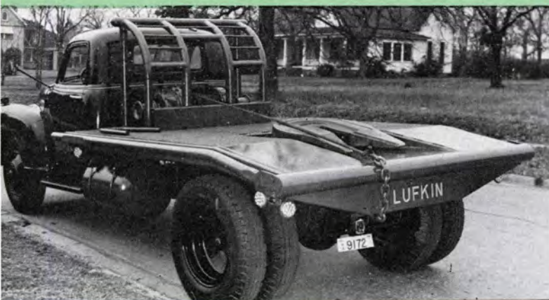
THIS MODEL MIGHT be referred to as a convertible. It can be used either as a single or tandem self-loading float, or as a single or tandem pipe trailer, or as a bed job for local purposes.
