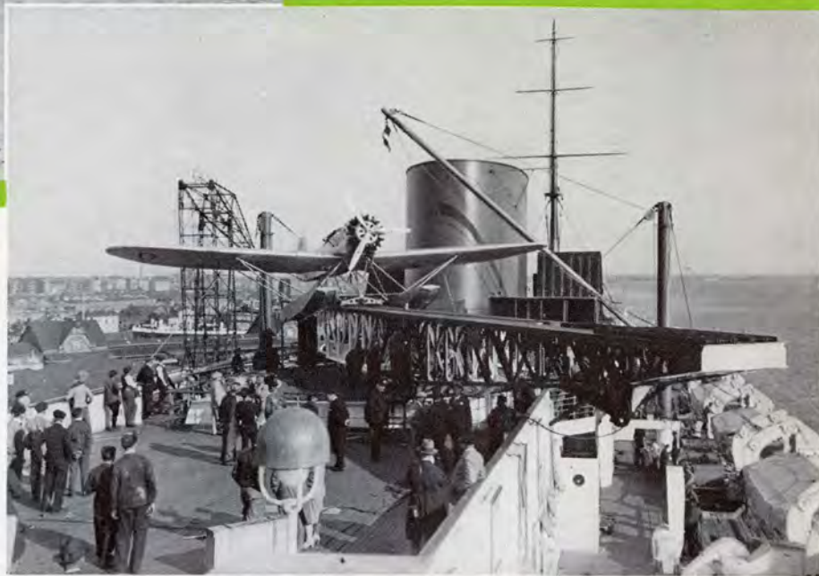
PASSENGER-SHIP CATAPULTS —Several of the speedy French and German liners are equipped with catapults for launching small planes that carry mail back to ports of departure or speed it to ports of destination in advance of the arrival of the ships. These pictures were taken on the "Bremen" and the "Europa."
