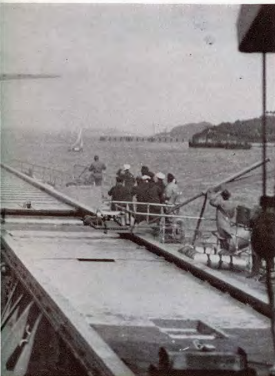
large ocean-mail flying boat on the runway of the catapult of the "Ostmark." In the foreground are the cables that draw the plane forward and, at either side of the central slot, the air-operated brakes that retard the progress of the carriage after the plane has taken off. Lower picture is a view from the opposite end of the same runway, showing a plane that has just been successfully shot out into space.
