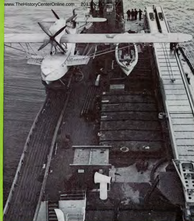
TAKING A PLANE ABOARD —The drawing illustrates the crane on the "Ostmark" lifting a plane aboard for servicing. The vessel is equipped with a wide canvas strip that can be unrolled and towed astern to serve as a ramp on to which a plane can be taxied in case the ocean is too rough to permit it to approach close enough to be picked up. The photograph shows a plane hoisted aboard the "Schwabenland" and placed on the turntable. The air-operated catapult which will launch it is shown at the right.
