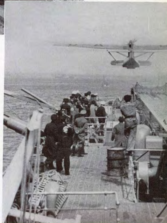
LAUNCHING A PLANE FROM A SHIP—The "Oostmark," which serves as a seaplane base on the German air-mail route between Africa and South America is pictured at the top of this page. The vessel is equipped with a derrick to lift planes aboard for servicing and refueling them, and with a catapult for launching them. It is 245 feet long and is powered by two oil engines. Center picture shows a
