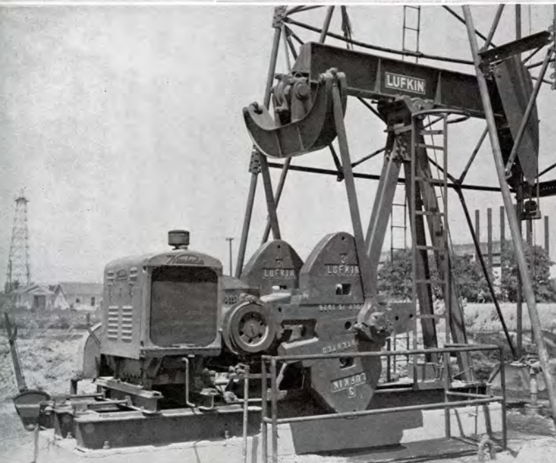
Amerada Oil Co., Walker Lease, Fittstown, Oklahoma, Lufkin TC 3-22C Unit Assembly.
