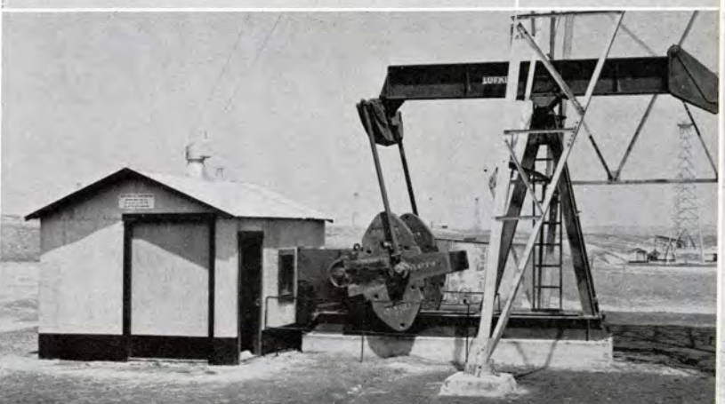
Deep Rock Oil Co., Lufkin TC 2A-26 Unit Assembly, Bemis Pool, Hays, Kansas
