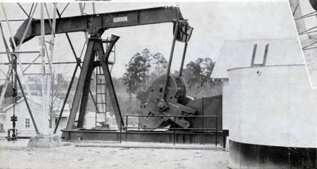
"Bow-legged?"—Not exactly. This is the LUFKIN No. 17A Jack on Hearrell & Burnett's Gladewater Well, which was partially submerged by the New Year's Day flood of the Sabine River.
