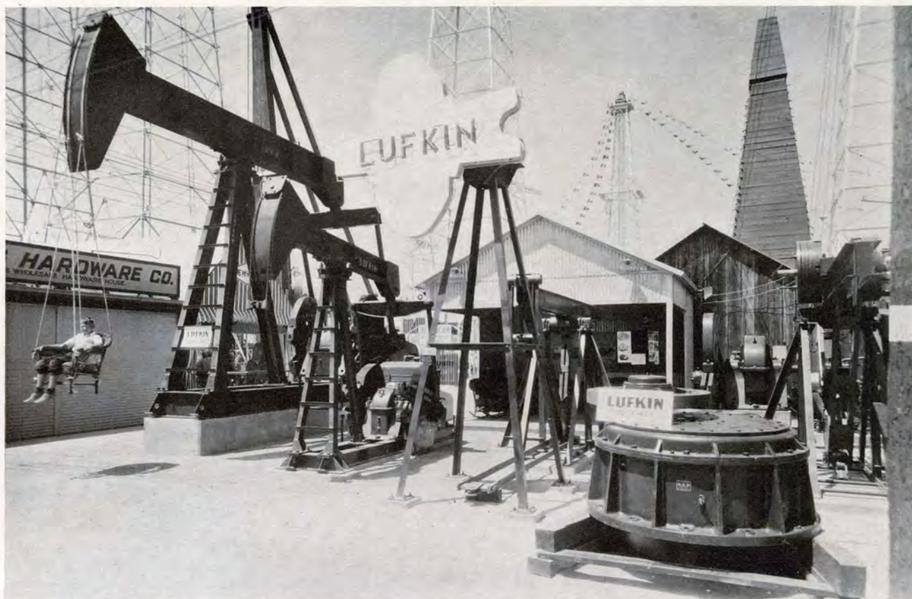
LUFKIN'S EXHIBIT AT THE TULSA OIL SHOW —Lufkin's Exhibit at the Tulsa show consisted of various sizes of pumping units in operation; Lufkin's herringbone central power, jacks and counterbalance take-off for "back-side" crank pumping. A feature of the exhibit was the chair attached to the horsehead of one of the larger type units which provided a "ride" and a thrill for many of the visitors to the Lufkin booth. Walter W. Trout, Assistant to the President of the Lufkin Foundry & Machine Co., in charge of the booth had his trusty kodak well stocked with films and exhibits of his work will be found on pages 8 to 11 inclusive.
