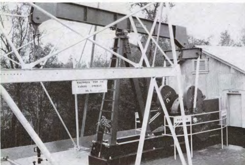
Lufkin T. C. 2-26 Pumping Unit. Superior Engine, Nadine Utzman No. 1, Magnolia Petroleum Co., East Texas.
