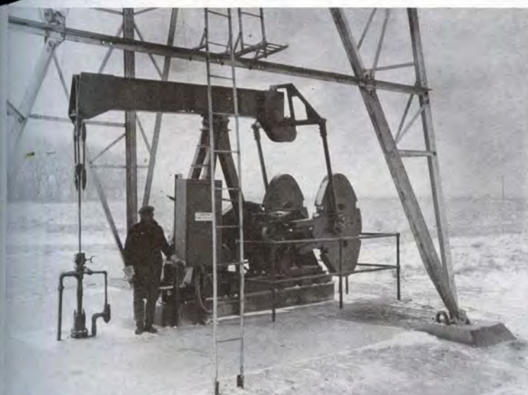
Lufkin T. C. 3-22 Pumping Unit, G. E. Motor drive, Stanolind Oil & Gas Company, Werrie No. 1, Ellenwood, Kansas, Ben Snyder, farm boss.
