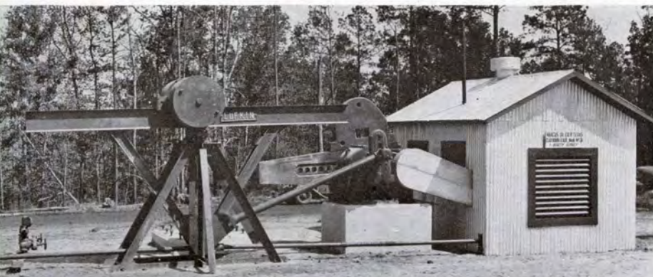
Lufkin No. 31 Unit with backside crank, counterbalance swing, Marcus Oil Company, Clayborn lease, well No. 3 Beatty survey, East Texas.
