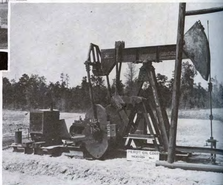
Lufkin T. C. 4-11 Pumping Unit with extra well take off, Perot Oil Corporation, Dickinson No. 1 Pena Survey, East Texas.
