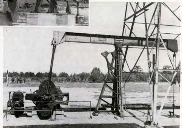
Lufkin No. 48 Herringbone Unit with Center-line Beam Assembly—Stanplind Oil & Gas Company, Cayuga District.
