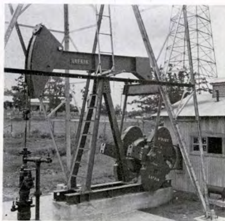
Lufkin No. 3-18 Twin Crank Unit complete assembly. Cherokee Chief Oil Company, Todd No. 1, Gladewater area.
