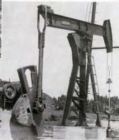
Lufkin No. 31 Double Reduction Herringbone Unit with Standard Post Assembly. Burwyn Oil Company, East London District.
