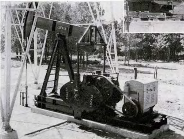
Lufkin Twin Crank Unit Assembly with structural base arranged for gas engine drive. Sinclair Prairie Oil Company, Laurther Lease.
