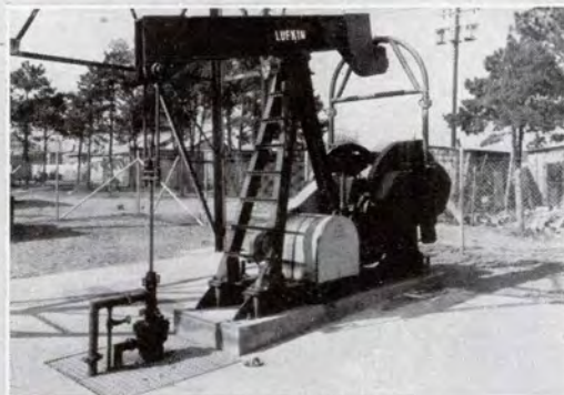
LUFKIN T. C. 6-11 UNIT ASSEMBLY WITH MOTOR MOUNTED UNDER SAMSON POST MAKING A VERY COMPACT ARRANGEMENT.
