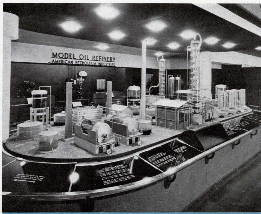
Model Refinery—One of the most interesting exhibits of the oil industry is located in the main room of the Hall of Science. Major refining operations, from the fractional distillation of crude oil to the final treatment of the five basic products and including the cracking process, are demonstrated in a glass-enclosed model refinery, extending 30 feet in length.
