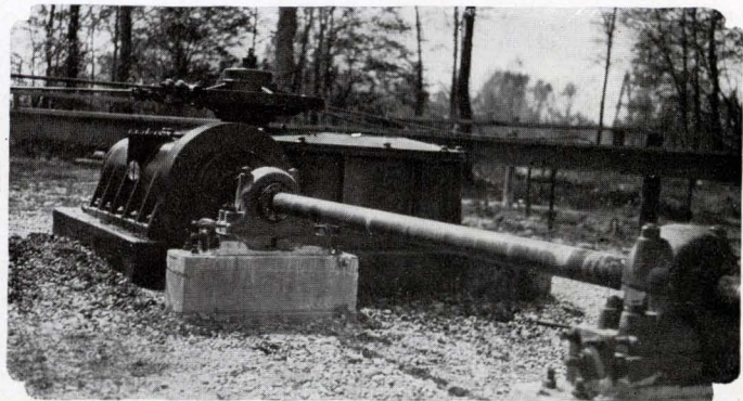
First geared pumping unit in East Texas—LUFKIN GIANT POWER on lease of H. L. Hunt Company, near Henderson.
