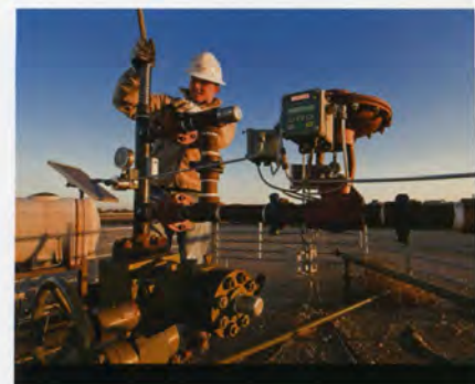
Plunger Lift Systems provide an economic artificial lift solution that uses residual well pressure to lift fluids to surface.
