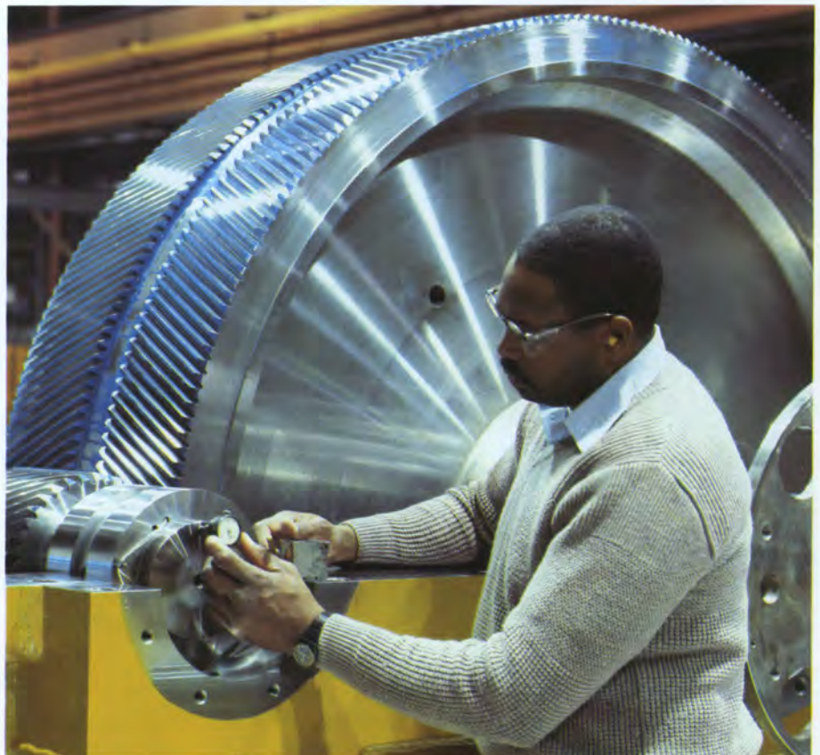
A technician checks shaft end play on a large high speed gear, rated for 35,000 horsepower.
