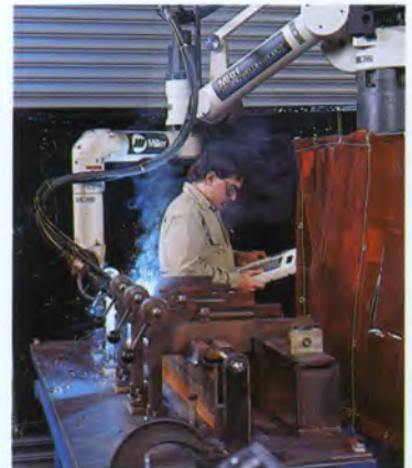
An automated welding device is used to weld small parts and assemblies for pumping units and commercial fabrication products.
