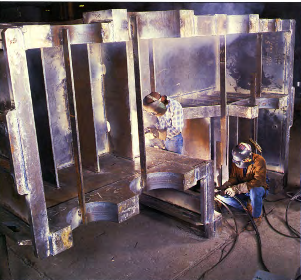
Left: This massive gear box will house a 4000 horsepower rubber mill gear drive which will be shipped to Korea for installation in a tire plant.
