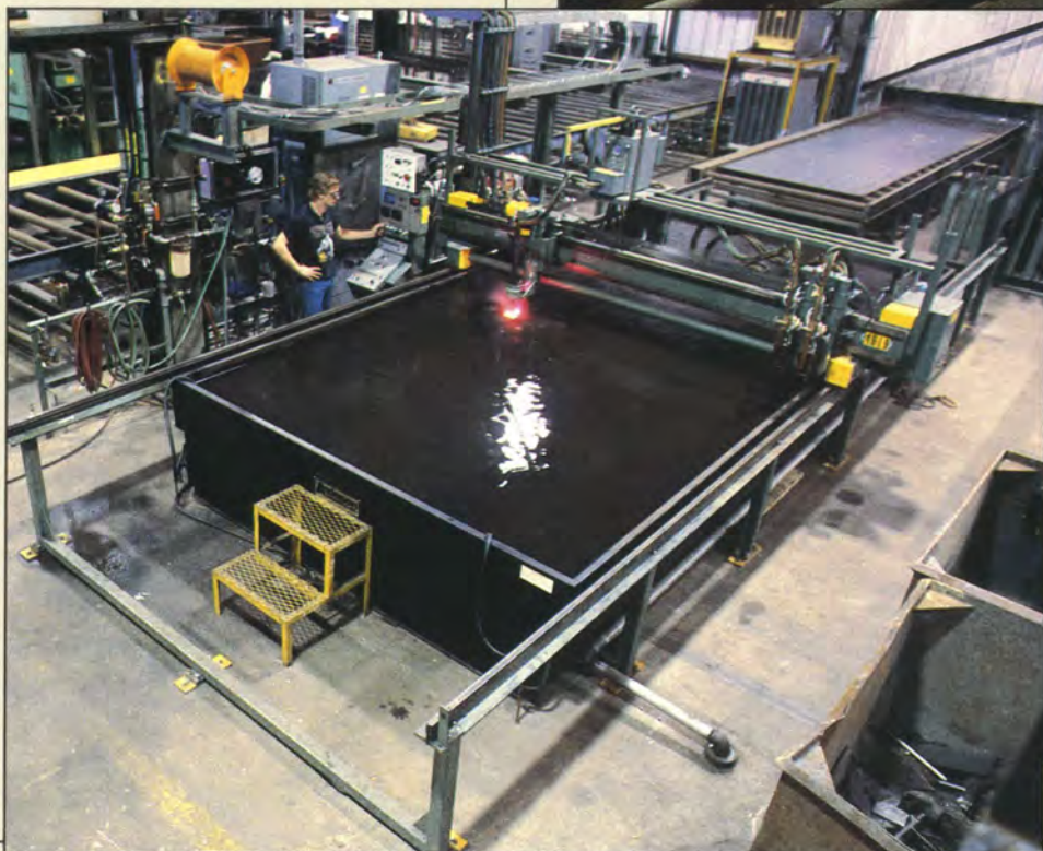
Above: A new plasma arc burning machine is an integral part of the walking beam factory. Right: Ductile iron gears are being poured in the new facility where production began in 1985
