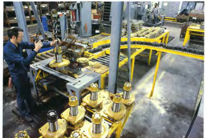
Conveyors, overhead lines bring parts for crank pin assembly
