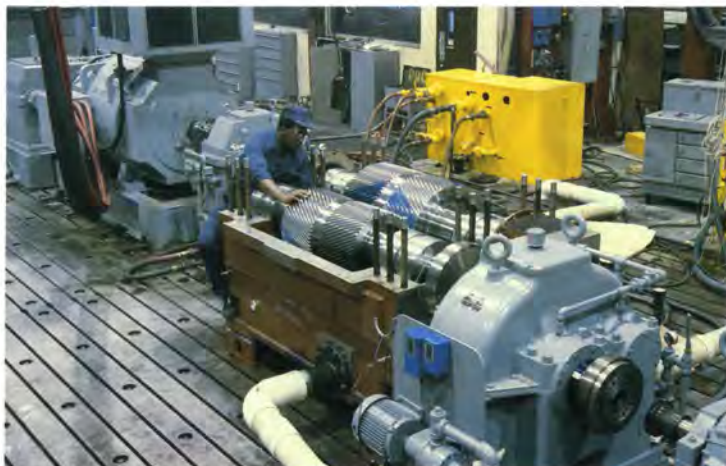
A 67,000 h.p. gear is largest ever built by LUFKIN
