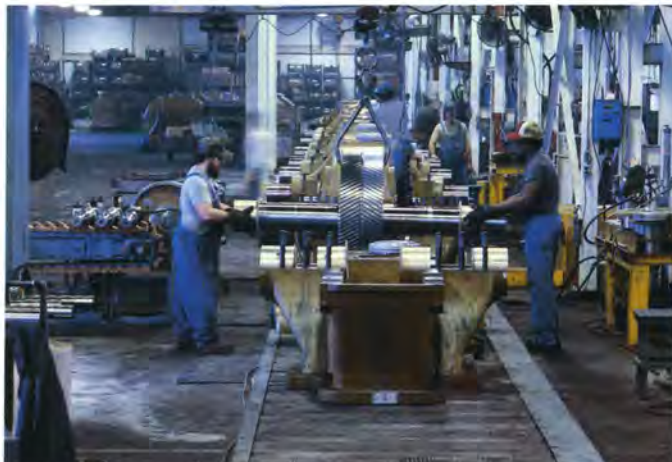
In the gear box assembly area, parts arrive by conveyors
