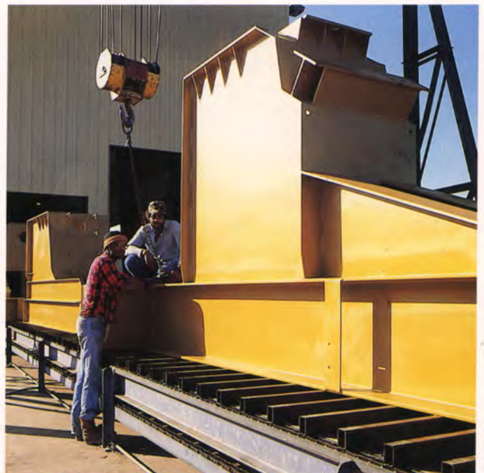
Mark II bases leave structural plant for final assembly
