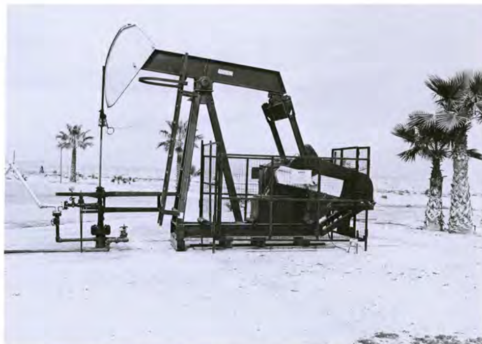
Called a “nodding donkey” by the oilmen of Oman, A LUFKIN pumping unit brings the heavy crude of Marmul to the surface.
