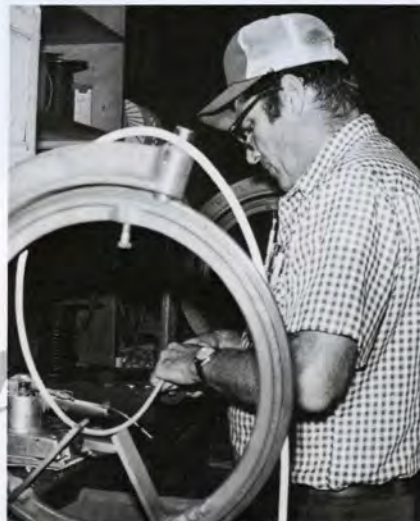
Don Jackson rewinds a motor in the electrical rewind area. The area is responsible for rewinding motors with damaged wiring.
