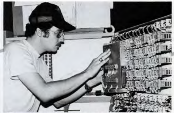
Electronics technician Michael Miles examines the control panel on a computer-controlled shaft grinder. The electronic technicians of the machinery group are responsible for installation and maintenance on all numerically-controlled machinery.
