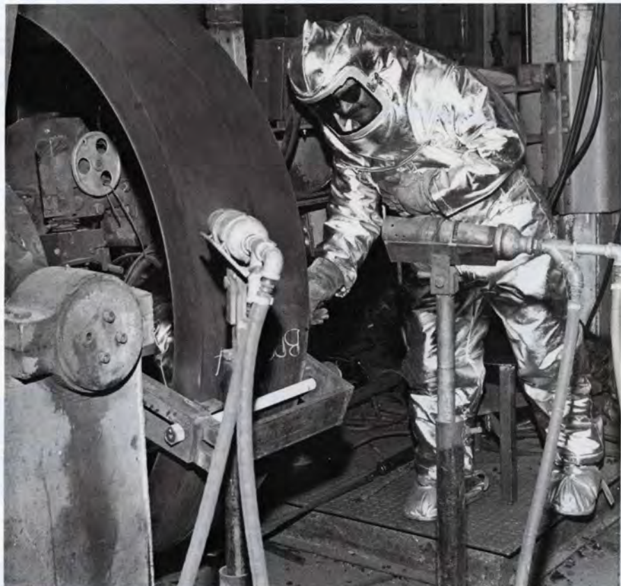
First shift welder Oscar Vasquez wears one of the new air-conditioned suits to protect himself from high temperatures while welding a gear rim.
