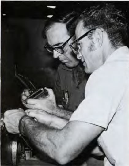
(l-r) Electronic technicians Mike Hartman and Joe Mac Pittman replace an encoder on a shaft grinder in the shaft shop. Technicians must know how to operate all machinery before they can effectively repair it.
