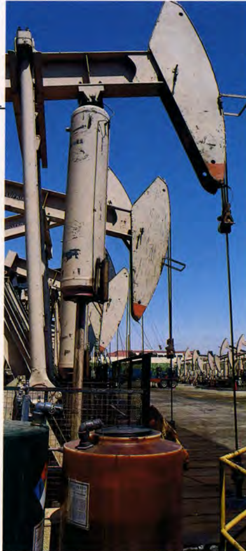
LUFKIN Air Balanced units were selected because of their economy and trouble-free operation.
